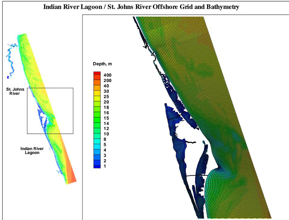
Figure 8. A horizontal numerical grid for Indian River Lagoon, St. Johns River, and a large coastal area.
