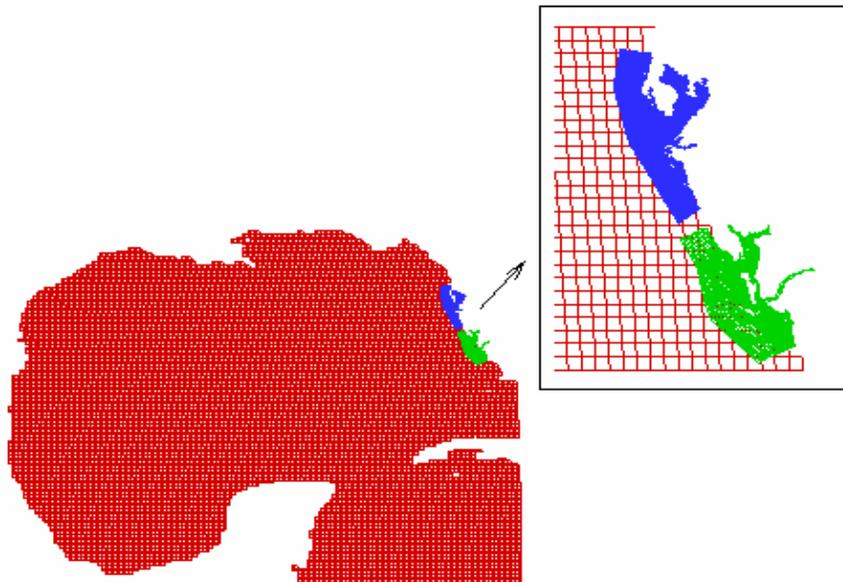
Figure 10. Numerical grids of Tampa Bay and Charlotte Harbor, which are coupled to a Gulf of Mexico grid.
