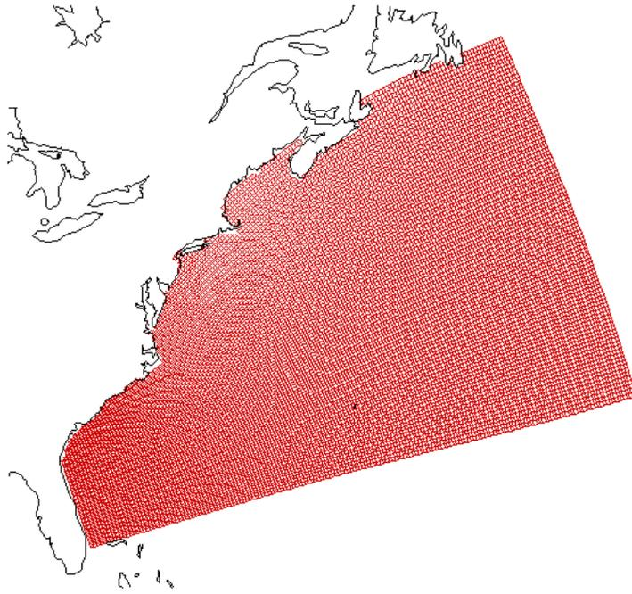
Figure 6. Numerical grid used by the NOAA Regional Ocean Forecast System (ROFS).
